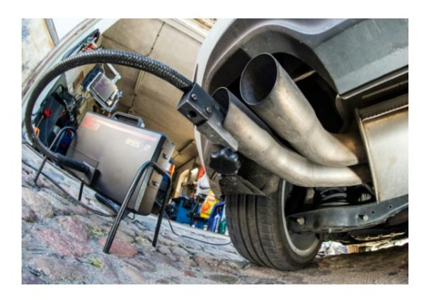
A measuring hose for emissions inspections in diesel engines in the exhaust tube of a Volkswagen Golf 2.0 TDI diesel car at a garage in Frankfurt an der Oder, eastern Germany, on October 1, 2015
