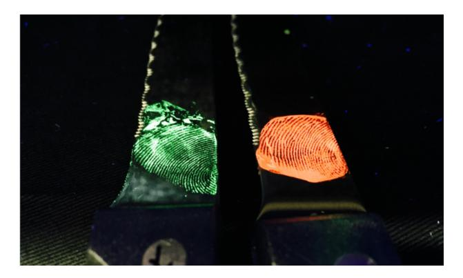
Different colours can be achieved by altering the chemistry of the solution. This photo shows the method on the blades of two knives.
