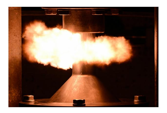
A small amount of explosive material is subjected to shock wave with a striker plate to induce detonation. An explosive material's insensitivity — its resistance to accidental or unintended detonation — is one set of data measured using this type of test. Credit: LANL photo by Daniel Preston
