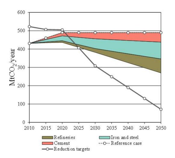
The colored fields (wedges) show estimated emission reductions achieved in the carbon-intensive industry in the period 2010–2050, assuming ambitious deployment of technologies and measures that are currently commercially available. Despite the extensive measures that are assumed to be implemented,
