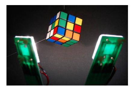
This image of single-doped organic light-emitting diodes (OLEDs) shining a high-quality white light on a Magic Cube shows how OLEDs can vividly illuminate the colors of the cube across the full range of the visible color spectrum from blue to green, yellow and red. ASU engineer Jian Li's research team is working to develop a cost-effective solution for the next generation of solid-state lighting products based on OLED technologies. Photo courtesy of Jian Li's research group.
