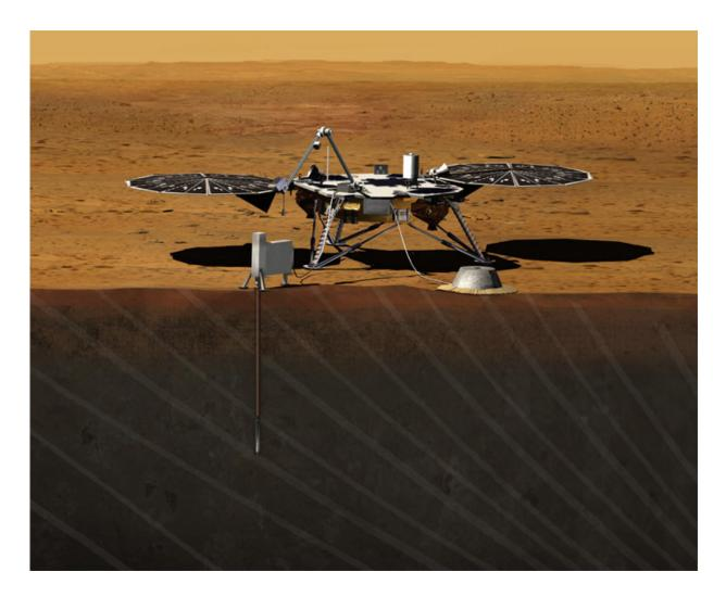
Artist rendition of NASA's Mars InSight (Interior exploration using Seismic Investigations, Geodesy and Heat Transport) Lander, which was selected as part of the Discovery Programs 2010 call for submissions and will be launched by 2016. Credit: JPL/NASA
