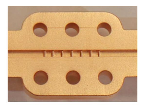
Cross-section of a 3D-printed split-block waveguide. Credit: Imperial College London
