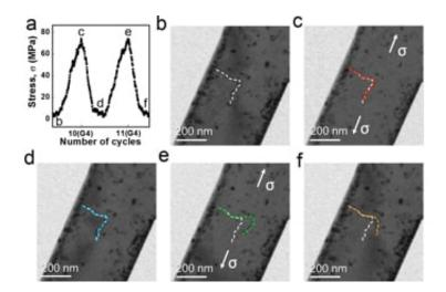
Abrupt de-pinning and de-stabilization of a dislocation line due to repeated cyclic loading. (a) Evolution of nominal tensile stress during two selected cycles: 10 and 11 in loading sequence G4, described in Table 1. Figures (b) to (f) are still frames extracted from the recorded movie that corresponds to the stress state marked in (a). The direction of tensile straining is indicated by the arrows in Figs. (c) and (e). The scale bars in (b) to (f) represent 200 nm.
