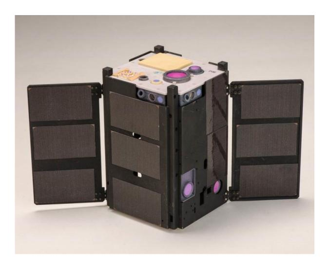
Optical Communications and Sensor Demonstration (OCSD) Spacecraft Configuration. OCSD differs from other space-based laser communication systems because the laser is hard-mounted to the spacecraft body, and the orientation of the CubeSat controls the direction of the beam. This makes the laser system more compact than anything previously flown in space. Credits:
