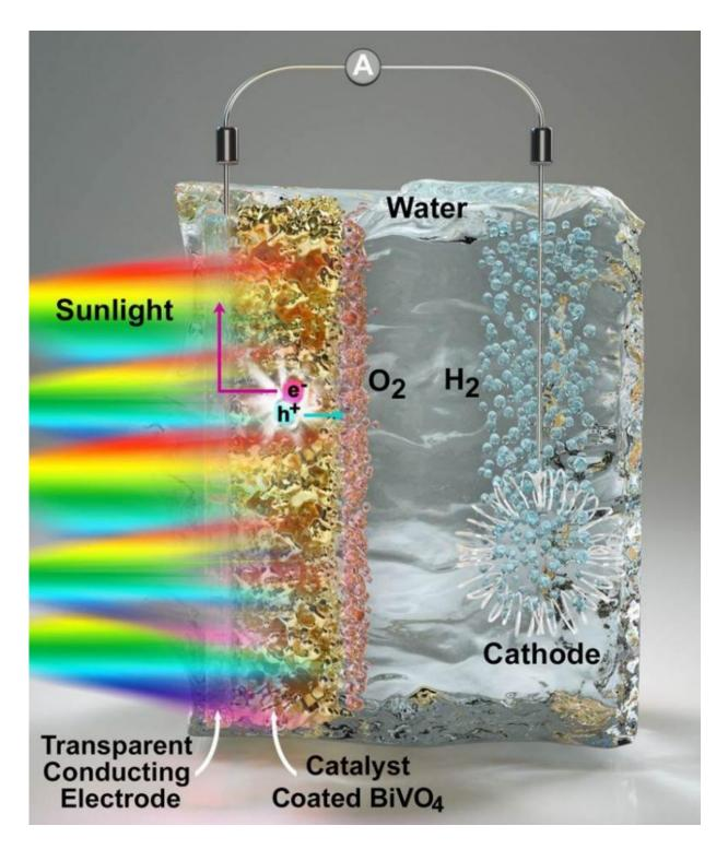
Splitting water into hydrogen provides a means of harvesting the hydrogen for fuel. This image depicts the water-splitting process in a light-sensitive electrode material (BiVO4), which UChicago and University of Wisconsin researchers investigated in an experimental and computational study. Credit:
