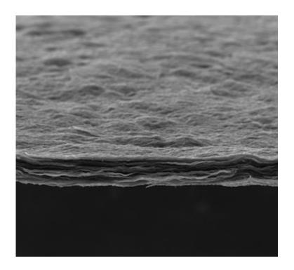
A new catalyst just 15 microns thick has proven nearly as effective as platinum-based catalysts but at a much lower cost, according to scientists at Rice University. The catalyst is made of nitrogen-doped graphene with individual cobalt atoms that activate the process. Credit: the Tour Group
