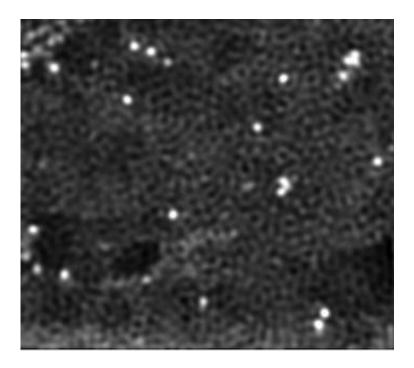
Cobalt atoms shine in an electron microscope image of a new catalyst for hydrogen production. Credit: the Tour Group
