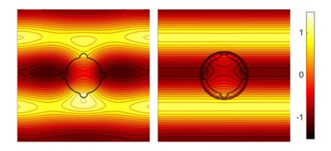
In a new twist, a team of researchers from the U.S. Naval Research Laboratory and the University of Texas at Austin has applied to acoustic waves the concept of "scattering cancellation," which has long been used to systematically cancel the dominant scattering modes of electromagnetic waves off objects.
