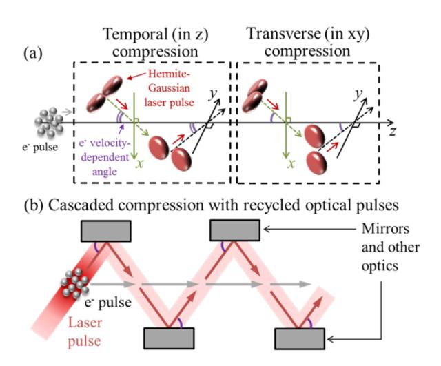
An all-optical, 3-D method of electron pulse compression for applications like ultrafast electron imaging is shown schematically in (a), with a cost-effective implementation depicted in (b). Credit: Liang Jie Wong/ Singapore Institute of Manufacturing Technology and Massachusetts Institute of Technology
