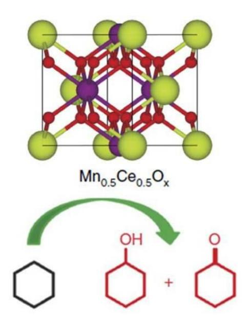
Oak Ridge National Laboratory's new catalyst is capable of selective oxidation of cyclohexane to cyclohexanol and cyclohexanone. Credit: ORNL
