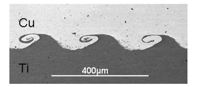
A microscope view of copper (top) welded to titanium (bottom) using a new technique developed at The Ohio State University. Credit: Glenn Daehn, The Ohio State University.
