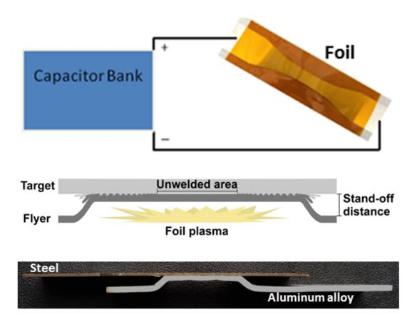
A diagram showing vaporized foil actuator welding, a technique developed at The Ohio State University. Credit: Glenn Daehn, The Ohio State University
