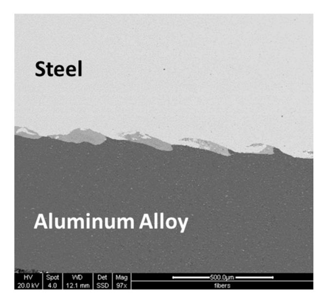
A microscope view of steel (top) welded to aluminum alloy (bottom) using a new technique invented at The Ohio State University. Credit: Glenn Daehn, The Ohio State University.
