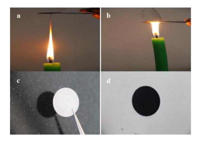
Collecting candle soot from the (a) tip of the flame and (b) middle of the flame. SS current collector (c) before and (d) after deposition of carbon soot. Credit: *Electrochimica Acta*, Volume 180 (October 2015), doi:10.1016/j.electacta.2015.08.124
