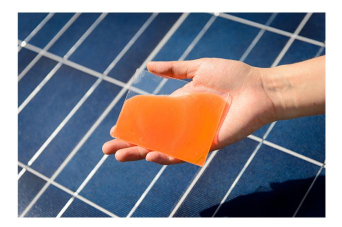
A gel developed by chemistry professor Challa Kumar that enhances the ability of solar cells to absorb energy from sunlight and could double the efficiency of existing solar cell panels. Credit: Peter Morenus/UConn Photo
