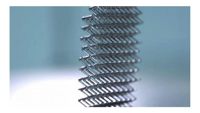
(Phys.org)—Airplane maker Boeing has unveiled what it calls the "The Lightest Metal Ever"—called microlattice, the material is a construct that is 99.99 per cent air. It has been developed by Boeing's HRL Laboratories along with colleagues at the University of California and the California Institute of Technology. The material has been developed as a way to reduce weight on airplanes or even rockets—a paper describing the development of the material was written by the team and
