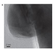
Optical black body, the fabrication of which occurs via seeded growth of Au nanospheres from Au nanorods. a, Low-magnification TEM image of a realized sample. b, TEM image of a single nanostructure. c, HRTEM image near the kissing point between the nanosphere and the nanorod. Credit: (c) 2015 *Nature Nanotechnology* (2015) doi:10.1038/nnano.2015.228
