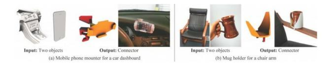
Want to mount a smartphone on your car's dashboard? On the arm of a chair? On your guitar? The choice is yours with a new method invented at Disney Research that automatically designs a custom connector that can then be produced with a 3D printer.
