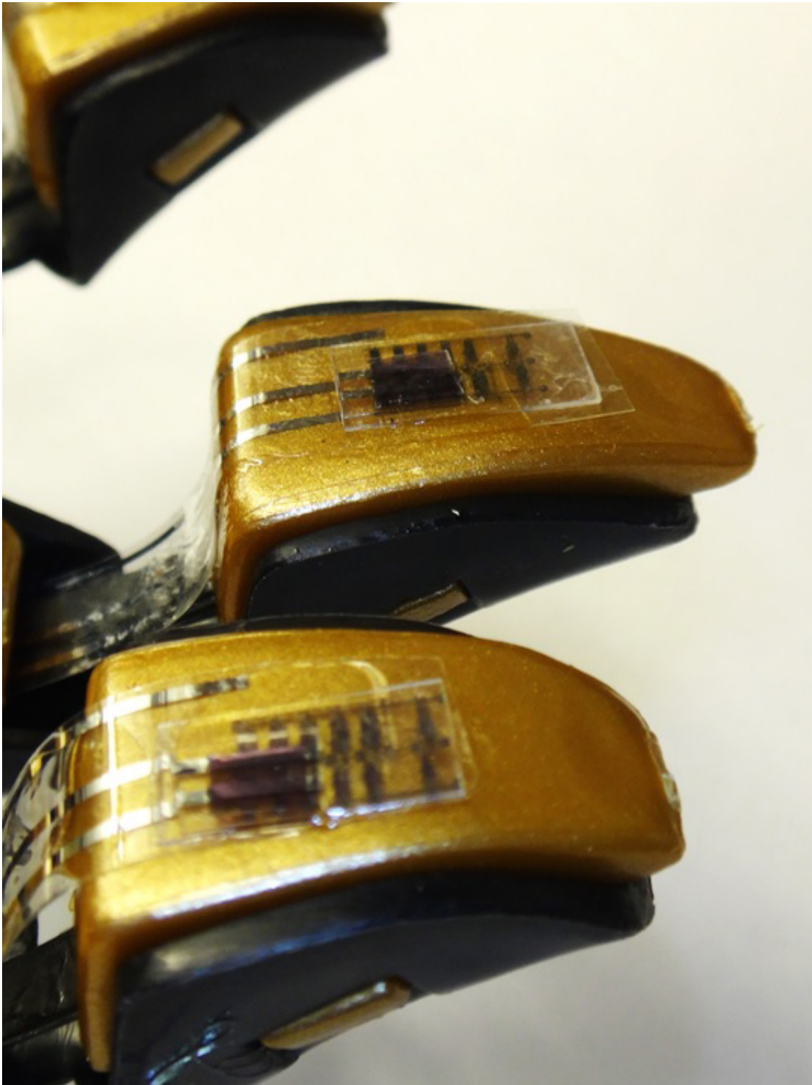
Artificial mechanoreceptors mounted on the fingers of a model robotic hand. Credit: Bao Research Group, Stanford University
