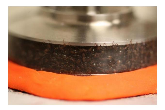
Ants were sheared in a rheometer, a machine used to test the solid-like and liquidlike response of materials such as food, hand cream or melted plastic.The researchers found that the behavior of live ants was similar to that of dead ants: when the aggregation is forced to flow, live ants let go and play dead. In this case, the viscosity dramatically decreased as the speed increased. Credit: Georgia Tech
