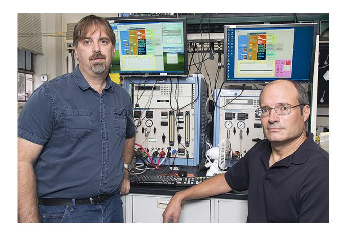
Rod Borup (left) and David Langlois simulate drive cycles on a fuel cell test station at Los Alamos National Laboratory to understand how carbon corrosion affects catalyst stability. Balancing durability and cost is a key challenge for the success of hydrogen-powered electric cars.
