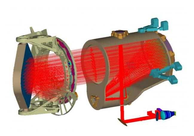
Optical ray tracing diagram of the Asteroid Impact Mission's laser-based optical communication terminal. The laser signal originates from the lens at bottom
