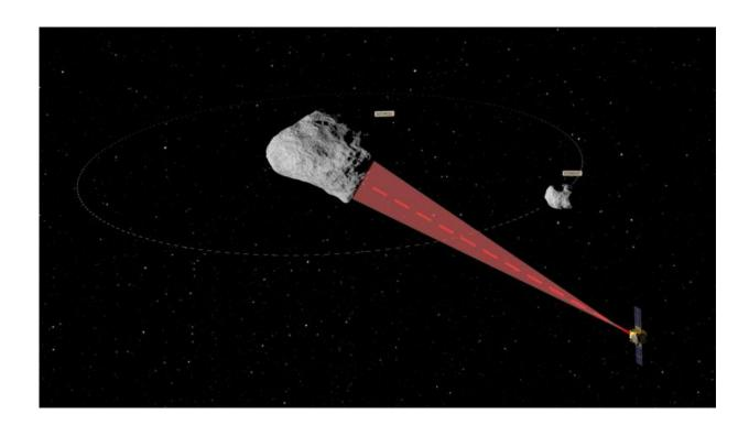
ESA's Asteroid Impact Mission will carry a powerful laser communication terminal to return scientific data to Earth. The laser can also be used for scientific purposes, such as laser altimetry to map the asteroid. Credit: ESA -
