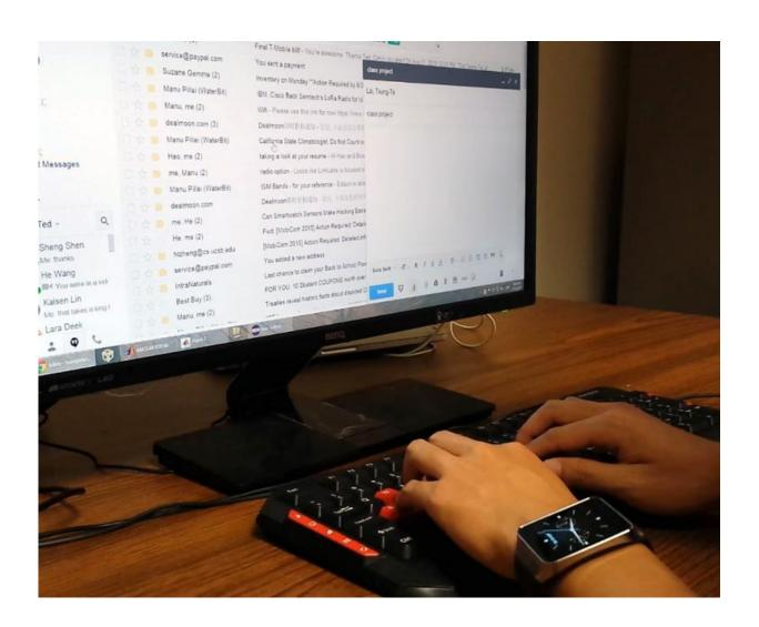
Using a homegrown app, researchers were able to guess what a user was typing through data 'leaks' produced by the motion sensors on smart watches. Credit: University of Illinois
