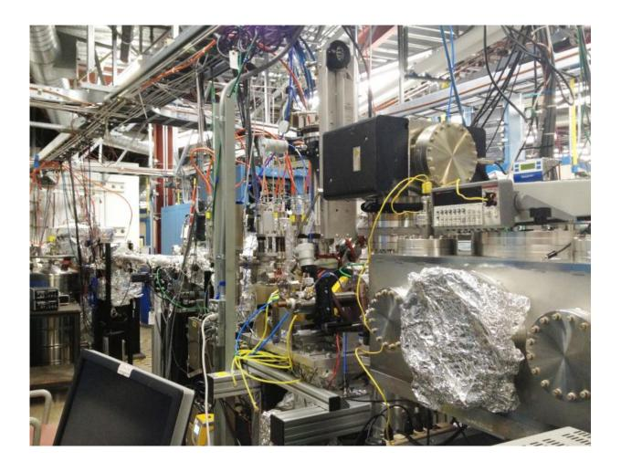
A scanning transmission X-ray microscope (STXM) at SSRL's Beam Line 13-1 that was used to observe a spin current relevant to spintronics. The microscope's vacuum chamber is on the right. Credit: SLAC National Accelerator Laboratory
