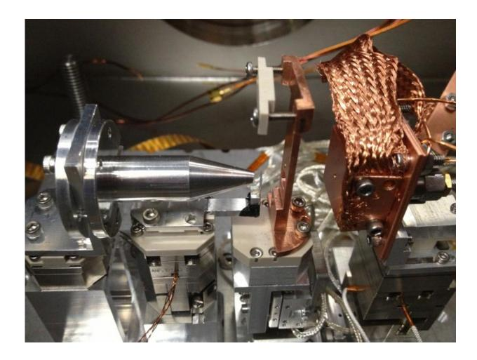
This microscope setup inside a vacuum chamber at SLAC's SSRL was used to observe a spin current relevant to spintronics. Credit: SLAC National Accelerator Laboratory
