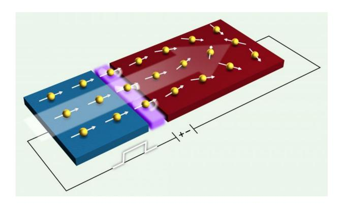
This illustration shows the flow of a magnetic property of electrons known as spin current from a magnetic material (blue), to a nonmagnetic material (red). Credit: SLAC National Accelerator Laboratory
