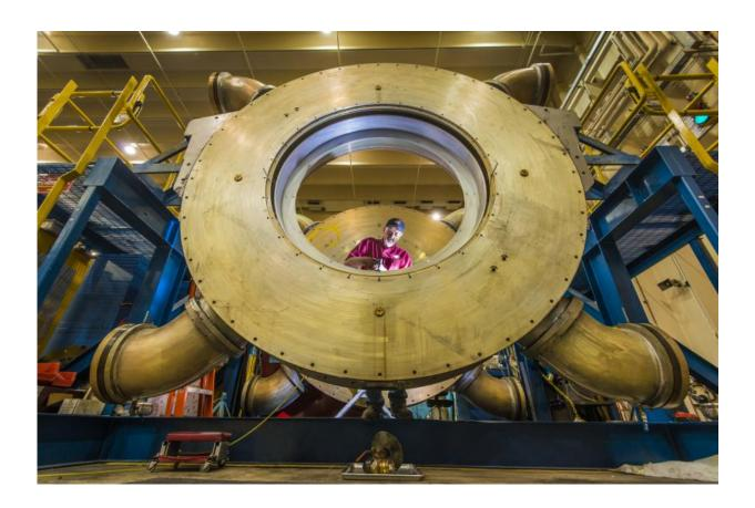
Technician Gary Tilley at Sandia Labs repairs a cavity at HERMES III. Credit: Randy Montoya
