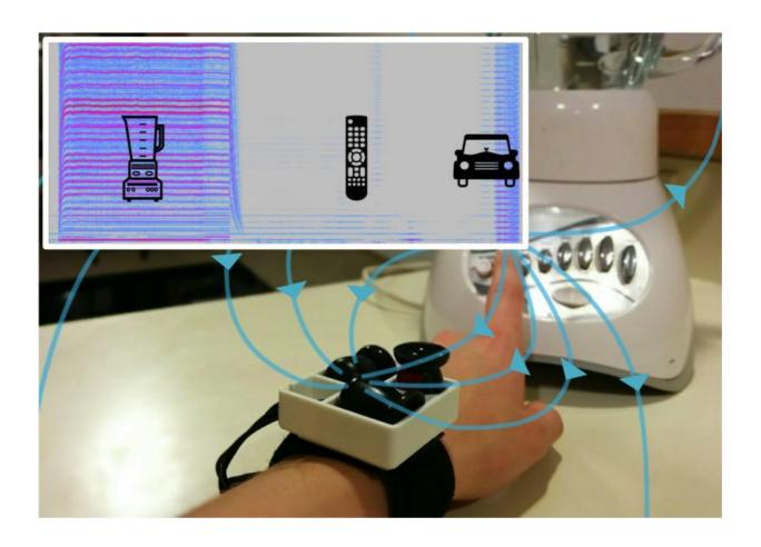
This MagnifiSense research prototype can sense what appliances its wearer is using, based on the electromagnetic radiation emanating from devices such as blenders, remote controls or even automobiles. Credit: University of Washington
