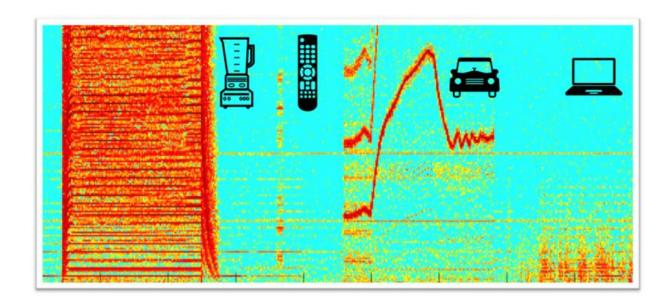
Appliances and vehicles such as cars, buses and trains emit a unique pattern of electromagnetic radiation, based on the combination of electrical components that make them run. Credit: University of Washington
