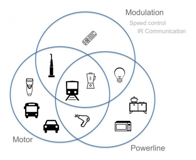
These sources of unique electromagnetic radiation patterns enable MagnifiSense to identify what devices its wearer is using. Credit: University of Washington
