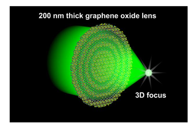
Researchers at Swinburne University of Technology, collaborating with Monash University, have developed an ultrathin, flat, ultra-lightweight graphene oxide optical lens with unprecedented flexibility.
