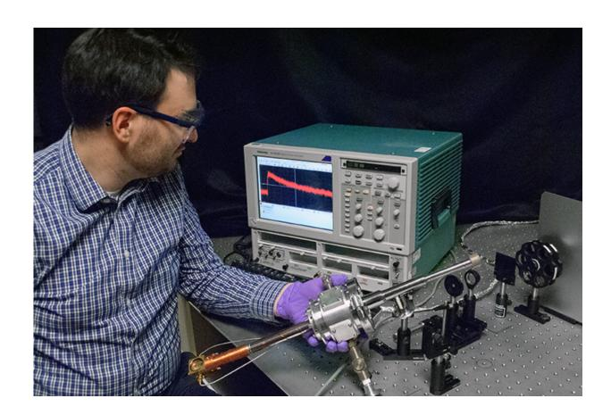
Andrew Fidler of Los Alamos National Laboratory examines an ultrafast photodetector used to measure quantum dot carrier multiplication in real time.
