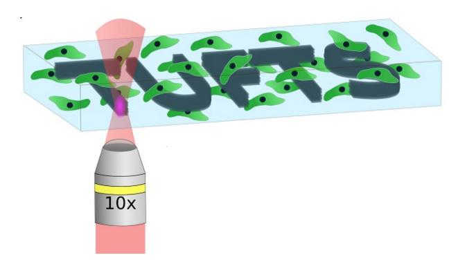
Illustration of laser-based micropatterning of silk hydrogels. The transparent gels enable the laser's photons to be absorbed more than 10 times deeper than with other materials, without damaging the cells surrounding the "Tufts" pattern. Credit: M.B. A
