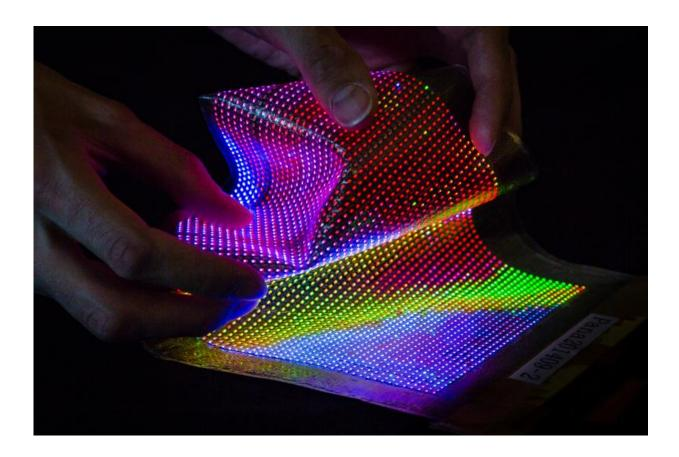
The world's first stretchable and conformable thin-film transistor (TFT) driven LED display laminated into textiles developed by Holst Centre, imec and CSMT.
