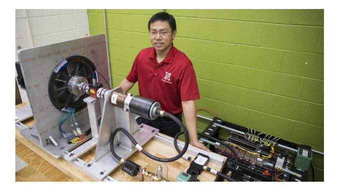
Jie Cheng, doctoral student in electrical engineering, stands next to the partial prototype of a wind turbine system that research suggests could yield 8.5 percent more electricity than conventional counterparts. Credit: Troy Fedderson/University Communications
