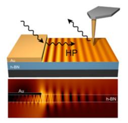
Illustration (top) and simulation (down) of nanoimaging slow nanolight in a thin boron nitride slab are shown. Incident light pulses are converted by a gold (Au) film into slow hyperbolic polariton (HP) pulses propagating in the boron nitride (h-BN) slab. The HPs are traced in space and time by first scattering them with a nanoscale sharp scanning tip and then measuring the time delay between scattered and the incident pulse as a function of tip position. Credit: CIC nanoGUNE
