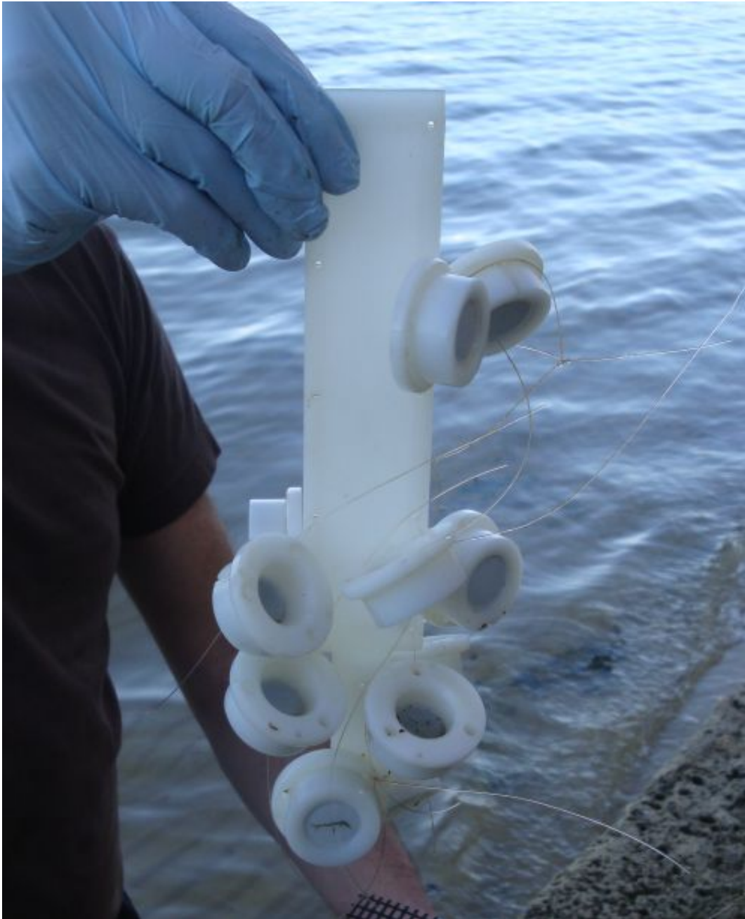
The collection devices which were used in the river. Credit: UWA
