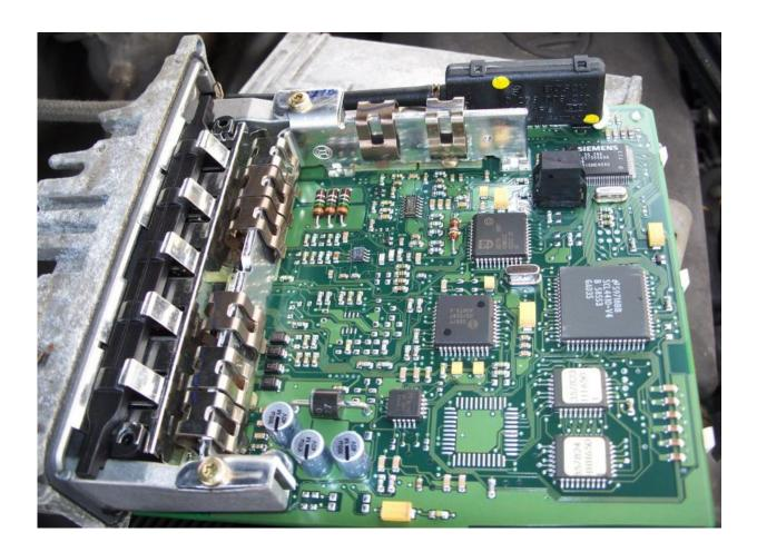
Interior view of a car computer for the Golf TDI motor controller. Credit: Wikipedia/Cschirp (CC BY-SA 3.0 DE)
