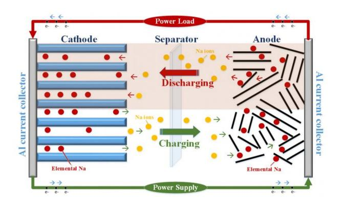
This schematic illustrates the functioning of sodium-ion batteries. The high cost and scarcity of lithium are driving research to develop alternatives to lithium-ion batteries, especially to meet future needs in energy storage. One potential alternative is sodium-ion batteries. Credit: Purdue University image/Vilas Pol
