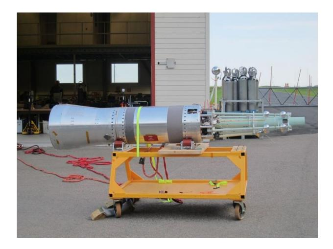
The forward section of the experimental rocket, showing several of the scientific instruments that will measure the dusty plasma. The silver spheres are part of the electric field instrument designed and built at the UW. After launch, they will
