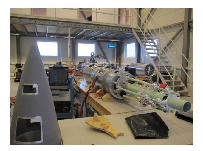
The forward section of the experimental rocket, right, showing several of the scientific instruments that will measure the dusty plasma. The rocket nosecone, which will cover the instruments during launch, sits at left. Credit: Todd Anderson
