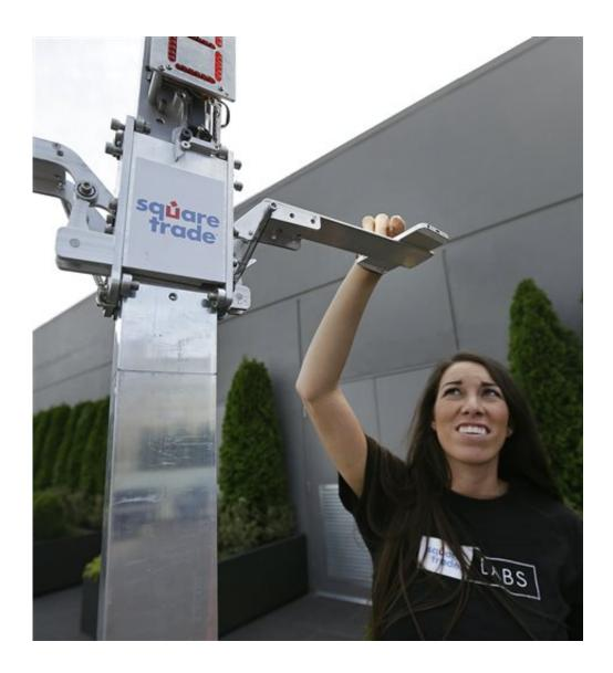
In this Aug. 26, 2015 photo, Chelsea Wickline, Associate Creative Director at SquareTrade, places a phone atop a DropBot, a robot used to test the durability of a phone, at SquareTrade offices in San Francisco. Despite engineering breakthroughs, screen breakage has become a part of life, the leading type of phone damage. (AP Photo/Ben Margot)
