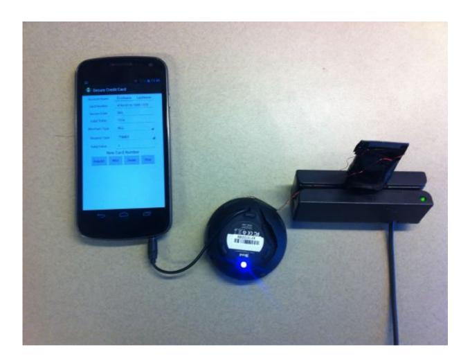
A picture of the "SafePay" prototype system (In real-world implementation,the amplifier and the solenoid can be combined together into one single chip,which can be directly plugged into the audio jack without a wire or connected with the phone through bluetooth). Credit: Yinzhi Cao, Xiang Pan, Yan Chen
