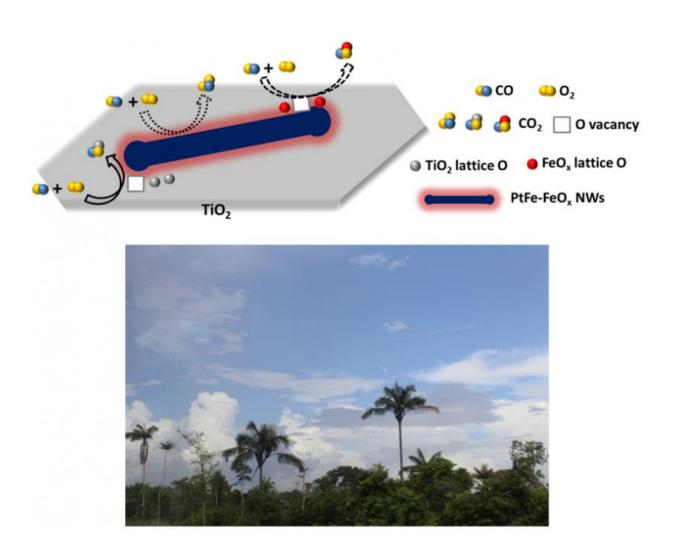
(Top) Schematic illustration of the two oxidation reaction regimes within the  $PtFe-FeO_x/TiO_2$  system. (Bottom) This new nanomaterials system could have a profound impact on the reduction of carbon monoxide pollution, improving air quality.
