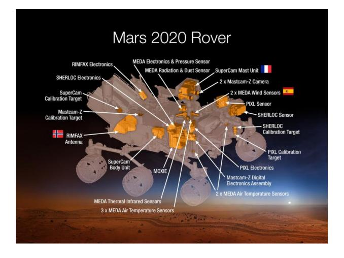
Science instruments on NASA's Mars 2020 Rover. Credit: NASA/JPL-Caltech
