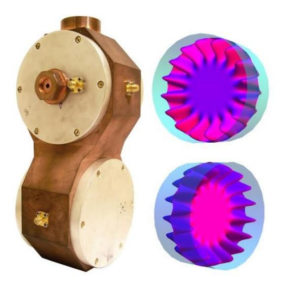
(Left) Photo of the orthogonal sapphire crystal mount, with (right) simulations of
