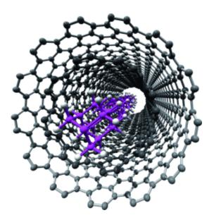
The inner space of carbon nanotubes can act as a template for the synthesis of nanodiamond-like carbon chains. As a team of scientists from Japan, Germany, and the United States report in the journal *Angewandte Chemie*, this templated polymerization approach paves the way for the design of novel one-dimensional nanomaterials.
