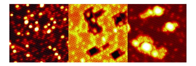
Left: Tiny platinum nanoparticles on an iron oxide surface. center: H2 gas leads to trenches in the surface. right: O2 gas causes additional iron oxide islands to grow.
