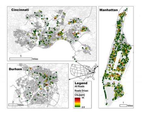
Maps of methane leaks surveyed in Cincinnati, OH (top left), Durham, NC (bottom left), and Manhattan, NYC, NY (right). Roads driven are outlined in darker gray, with leak locations marked by colored circles for methane concentration. Credit: Rob Jackson
