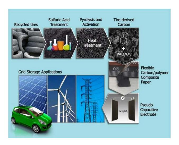
Instead of ending up in landfills, old tires can supply a key ingredient for supercapacitors to help power the nation. Credit: ORNL
