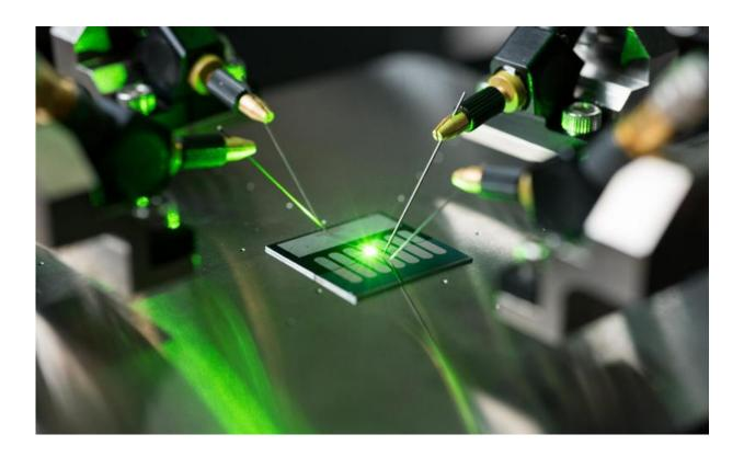
A carbon nanotube optical rectenna converts green laser light to electricity in the laboratory of Baratunde Cola at the Georgia Institute of Technology. Credit: Rob Felt, Georgia Tech
