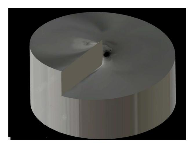
A schematic phase plate for imparting extra quantum units of orbital angular momentum. Neutron waves fall on the face of this plate, made by milling a dowel of aluminum into a ramp-shaped spiral. The steeper the pitch of the milled phase plate, the more orbital angular momentum will be imparted to the neutron beam. Credit: Ivar Taminiau
