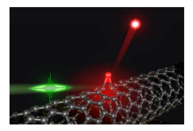
A solitary oxygen dopant (red sphere) covalently attached to the sidewall of the carbon nanotube (gray) can generate single photons (red) at room temperature when excited by laser pulses (green).
